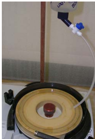
Drip system & whetstone wheel on Lap-Sharp™
