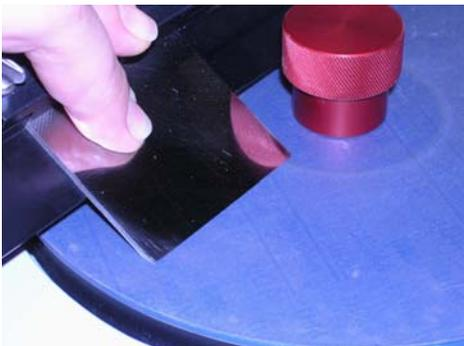
Plane Iron with polished back held in self squaring clamp and against the tool guide bar to sharpen the bevel edge.
