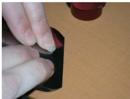
Japanese Plane Iron hand held on abrasive surface while sharpening the bevel edge.
